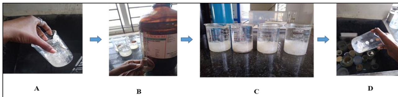
Fig 4: Hydrolysis-A-Washed FS with distilled water after pretreatment, B-Prepare 0.5M of HCl solution, C-FS treated with HCl solution for three days, D-Washed FS with distilled water after hydrolysis.
