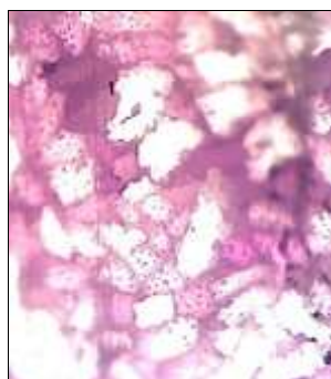
Cross sectional view of the semal fibres
