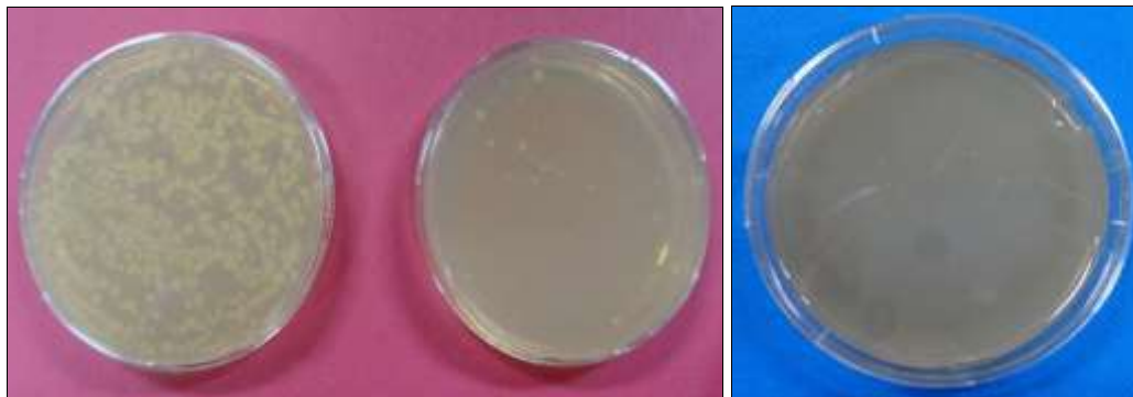
Fig 1: a. Photographs of Controlled sample, b. Only Neem treated c. Scoured & Neem treated samples
