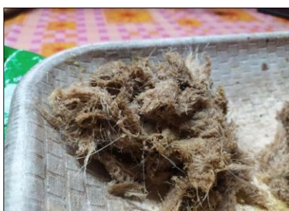
Fig 2: Processed banana stem fibres
