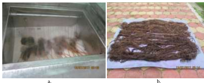
Fig 3: a) Degumming of Odal fibre b) Degummed Fibre
