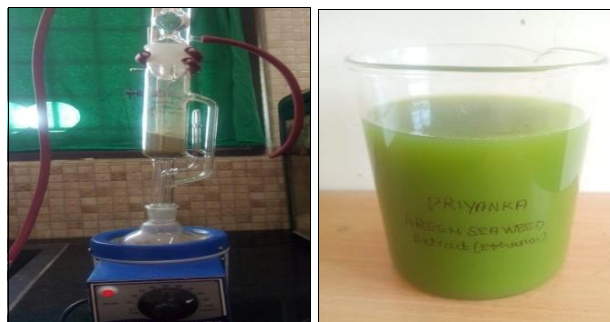
Fig 2: Soxhlet Extraction and Ethanol Extracted Solution
