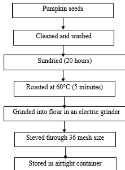
Fig 6: Flow diagram of processing of pumpkin seeds
