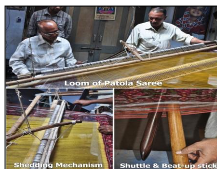
Fig 2.6: loom for making patola
