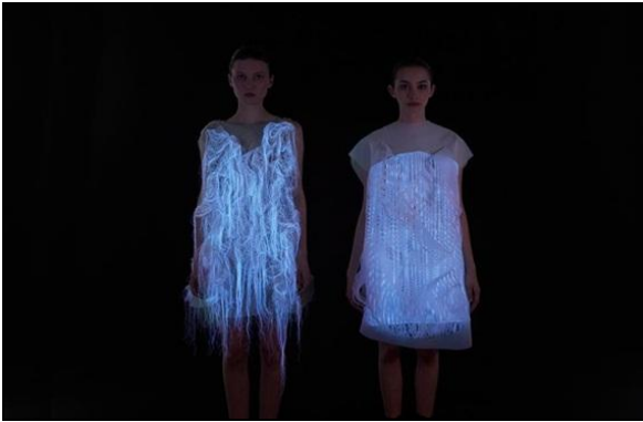
Fig 3: Dresses made from photo luminescent thread and embedded eye tracking technology from Ying Gao
