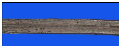
Fig 1: Longitudinal view of control muga silk fibre
