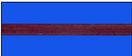
Fig 4: Longitudinal view of muga silk fibre printed with acid dye
